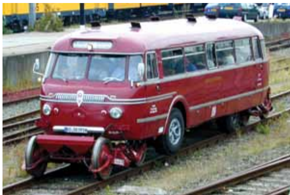
Example of a Hi-Rail vehicle from the Netherlands Photo: BSC/Arcadis
